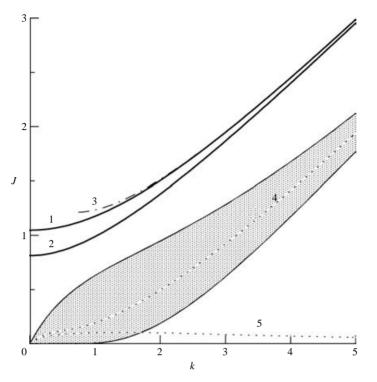
FIGURE 1. Instability domains for flows without inflection points on the velocity profile. The instability domain of the flow (1.2) is shaded. Curve 1, the upper boundary  $J = J_1(k)$  of the instability domain for the flow  $u = \tanh y$ ; 2, as curve 1 but, for  $u = 1 - e^{-y}$ ; 3, the WKB approximation of curve 1; 4, the line at which the growth rate in the flow (1.2) takes its maximum in J; 5, as curve 4 but, in the flow  $u = \tanh y$ .
