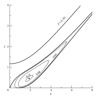
FIGURE 8. Instability domain of the flow with the piecewise linear velocity profile (1.2). Thin lines show contours of constant growth rate. The cross indicates the point of maximum growth rate ( $\gamma = 0.1233$  at k = 1.87 and J = 0.448).
