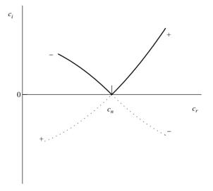
FIGURE 4. Trajectories of c(J) near the neutral curve when D(k) = 0. Signs near the lines designate the sign of difference  $(J - J^{(n)}(k))$ .
