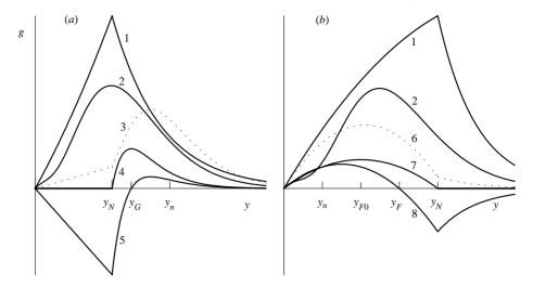
FIGURE 2. Eigenfunctions of neutral oscillations corresponding to the NCP  $y = y_n$  when (a)  $y_N < y_n$ , and (b)  $y_N > y_n$ . Curve 1,  $k > k_n$ ; 2,  $k = k_n$ ; 3,  $k_G < k < k_n$ ; 4,  $k = k_G (J = \infty)$ ; 5,  $0 < k < k_G$ ; 6,  $k_F < k < k_n$ ; 7,  $k = k_F (J = \infty)$ ; 8,  $0 < k < k_F$ . Dots show the eigenfunctions in unstably stratified (J < 0) flows.
