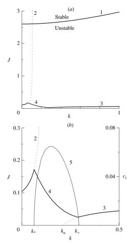
FIGURE 6. Instability domain of the flow (4.8): (a) the (k, J)-diagram; (b) lower part of the diagram (enlarged). Curve 1, the upper boundary of the instability domain  $J = J_1(k)$ ; 2, the long-wavelength branch of neutral oscillations; 3, their short-wavelength branch; 4, oscillations with  $c_r = c_n$  and  $k_* < k < k_+$ ; 5, dependence of  $c_i$  on k for these oscillations. Dots show the arcs of the curves 2 and 3 on which D(k) < 0.
